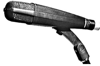
Sennheiser MD-421 dynamic cardioid [30-17 kHz]
